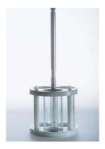
"B" Basket, (Test "B" 2.9.1.2 EP) 33 mm diam., used to test bigger samples order no. 101-2014 incl. glass tubes and disks
